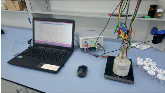
**Figure 1.** Potentiometric Measurement System
