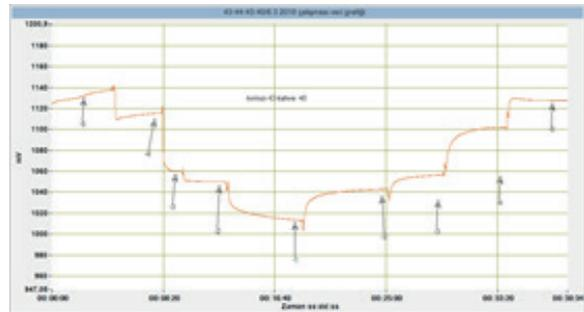
**Figure 4.** Stagnant environment measurements of the electrode numbered as 40 in  $1,0 \times 10^{-1}$  M and  $1,0 \times 10^{-5}$  M concentrations of NaCl and borate solutions.
