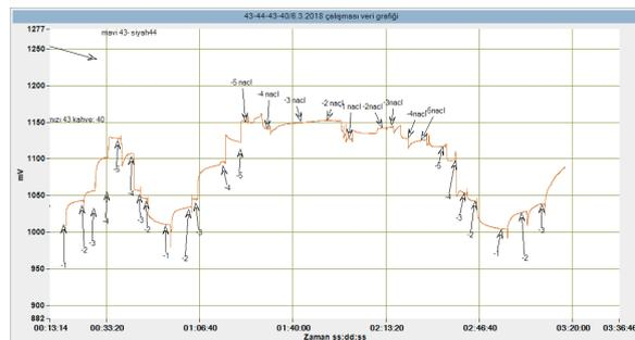
**Figure 5.** Stagnant environment measurements of the electrode in  $1,0 \times 10^{-1}$  M and  $1,0 \times 10^{-5}$  M concentrations of NaCl and borate solutions.
