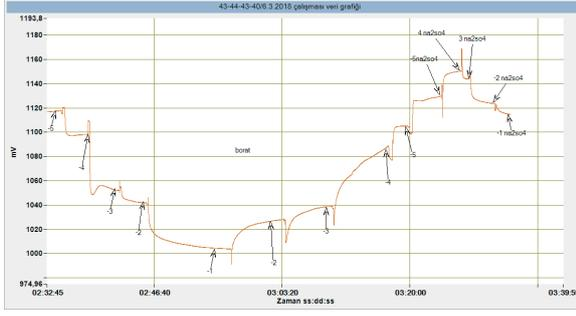
**Şekil 6.** Stagnant environment measurements of the electrode in  $1,0 \cdot 10^{-1} \text{M}$  and  $1,0 \cdot 10^{-5} \text{M}$  concentrations of NaCl and Na<sub>2</sub>So<sub>4</sub> solutions.
